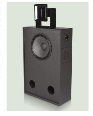
This is an improved (with SCD, screen compensation device) version of our well known LW 1003, with the bass and treble sections enhanced. Two way shalow cabinet screen system with crossover inside, very compact. 1x15" bass speaker and a 1,75" PM4 voice coil driver with external aiming device. For small cinemas up to 1300 m3.
